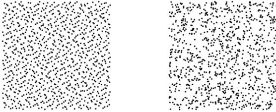
Fig. 6. 10^3 2D Halton points generated by Halton(2,3) (left) and 10^3 2D random points with uniform distribution (right).
